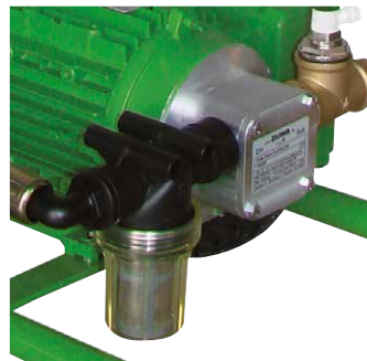
Pump with filter
