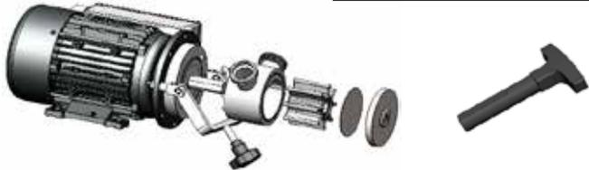
Remove the housing with the impeller, then press out the impeller or use the special tool for changing the impeller.
