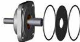
4. Remove O-rings and rear wear plate (with whole).
