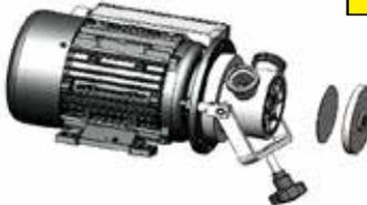
Release safety screw, lower bracket, remove front cover and front wear plate.
