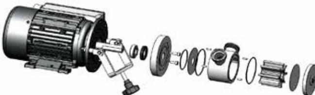
Remove the rear wear plate and the screws of the cylinder head, remove the cylinder head itself and withdraw the mechanical seal
