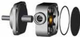
3. Remove wear plate (without hole) and housing with impeller.
