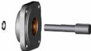
5. Detach locking ring and press out shaft.
