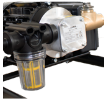
Pump with filter
